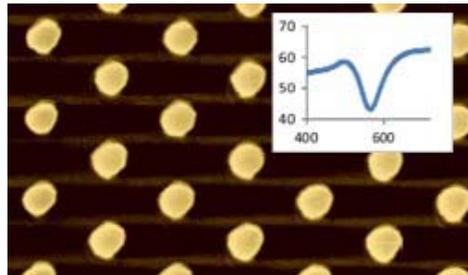
Spectrometric transmission measurements show a clear resonance at a wavelength of about 550 nm. The plasmonic structure is immediately available as an off-the-shelf standard product.
